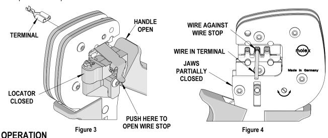
Open the tool by squeezing the handles together, at the end of the closing stroke, the ratchet mechanism will release the handles, and the hand tool will spring open.
